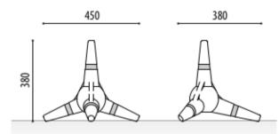
Alpes model road tetrapod made of highly flexible polyethylene plastic, which allows them to withstand large impacts and degradation from sunlight.
