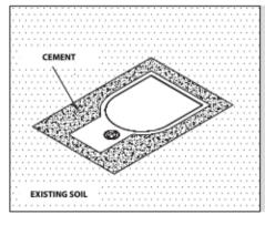
4. Level and fix the base correctly with cement.
