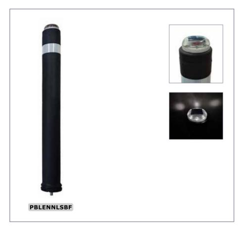
**A-Blen flexible luminous bollard with solar led beacon on the top,** the A-Blen flexible bollards are made of polyurethane plastic, after receiving an impact they return to their original shape and position. Easy installation by means of its screw-on system with a single screw to be screwed to the pavement, without losing the characteristics of the bollard.
